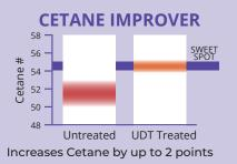
Increasing the cetane number improves fuel combustion, reduces white smoke on start-up, and tends to reduce NOx and PM emissions.
